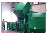
.Mark-Costello provides a heavy duty cart dumper to transfer treated waste from sterilizer cart to waste compactor. Hydraulic cart dumpers can be stationary mounted adjacent or integral to the compactor. Depending on the sterilizer model and cart size-either a stationary or self-contained compactor will be utilized.
