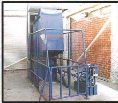
End load carriage dumper with one cubic yard tilt hopper dumping into load chute.
