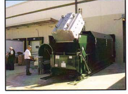
End load fork dumper dumping high volume autoclave carts into self-contained compactor.
