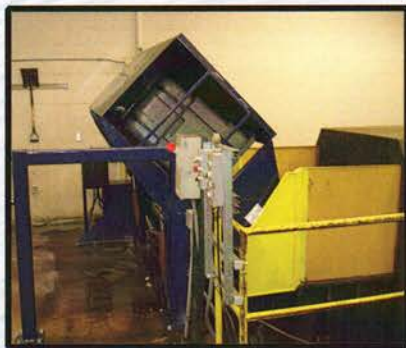
Side load carriage dumper with one cubic yard tilt hopper-dumping into self-contained compactor.
