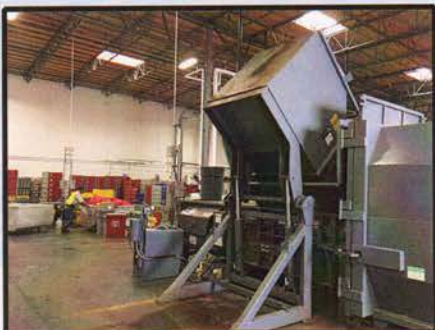
Side load carriage dumper dumping high volume autoclave carts into stationary compactor.
