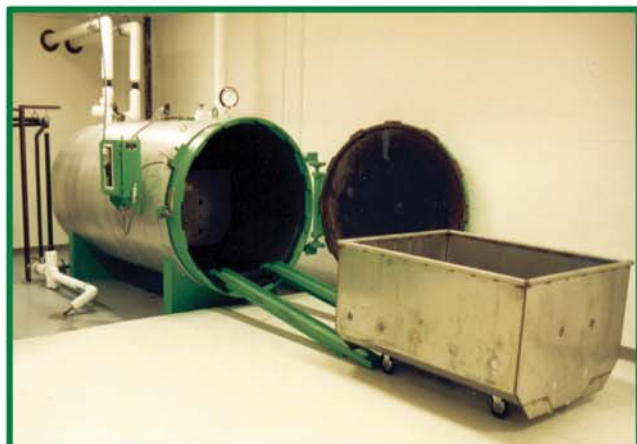
Equipped with optional cart ramp this AS510 installed at a Regional medical center allows carts to be easily loaded into sterilizer.
