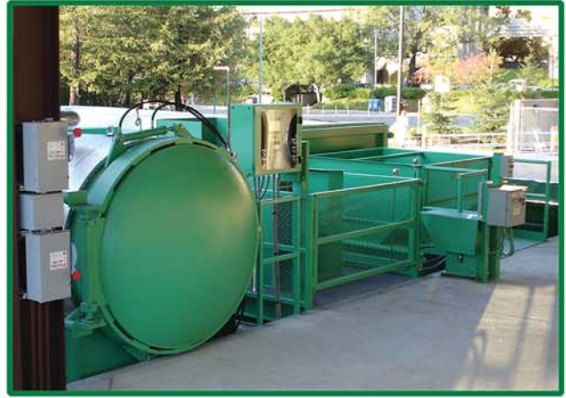
AS510 with vacuum and touch screen controller installed at dock with self-contained compactor for waste and stationary compactor for OCC.
