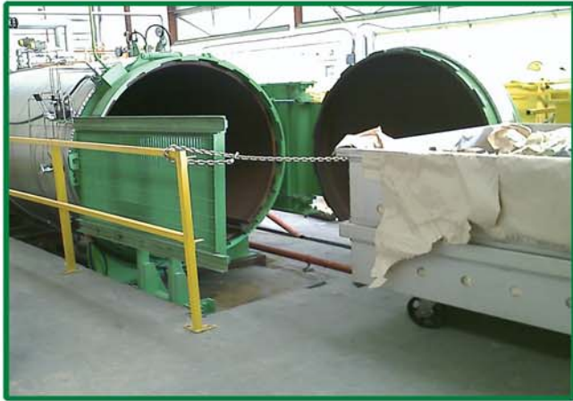
AS621DD (Double Door) w/Steam Jacket and vacuum pit-installed at a commercial waste processors plant utilizes optional hydraulic draw bridge to load carts.
