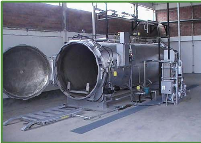
Installed at an International Airport-our model AS515 Hi-Volume/Stainless with vacuum treats international flight waste seven days a week-24 hours per day.
