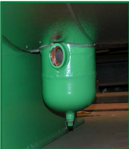
Front Mounted Sump Drain
