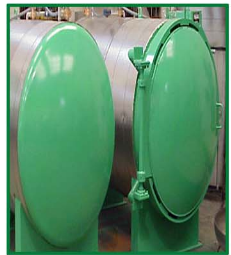
Fully Insulated Vessels Featuring Front and Rear Protective Steel Plates
