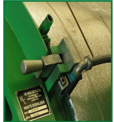
Door Lock With Quadruple Safety Mechanism
