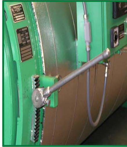
Ratchet Handle For Easy Lock-Unlock of Door Ring
