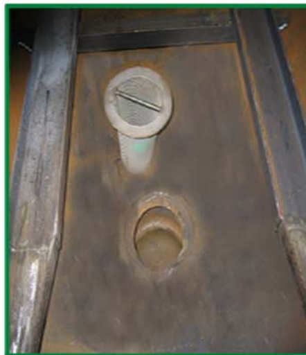
Internal Stainless Steel Basket Strainer For Front Mounted Sump Drain
