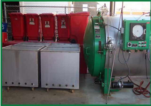
Equipped with optional hydraulic door lock-this large Eastern regional hospital, utilizes this AS47 to facilitate total on site Regulated Medical Waste management.
